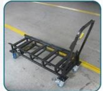
Push-pull type battery loading
